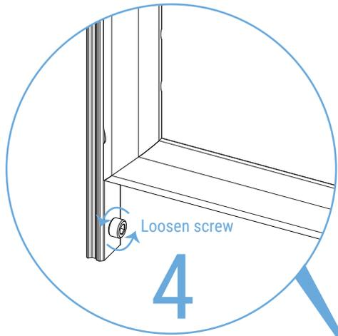
Loosen end block screws on panel.
