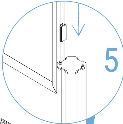
Install the panel into the posts with 2 people. Space posts 45.25" apart. With one person on each end of panel, guide panel end blocks into post grooves.
