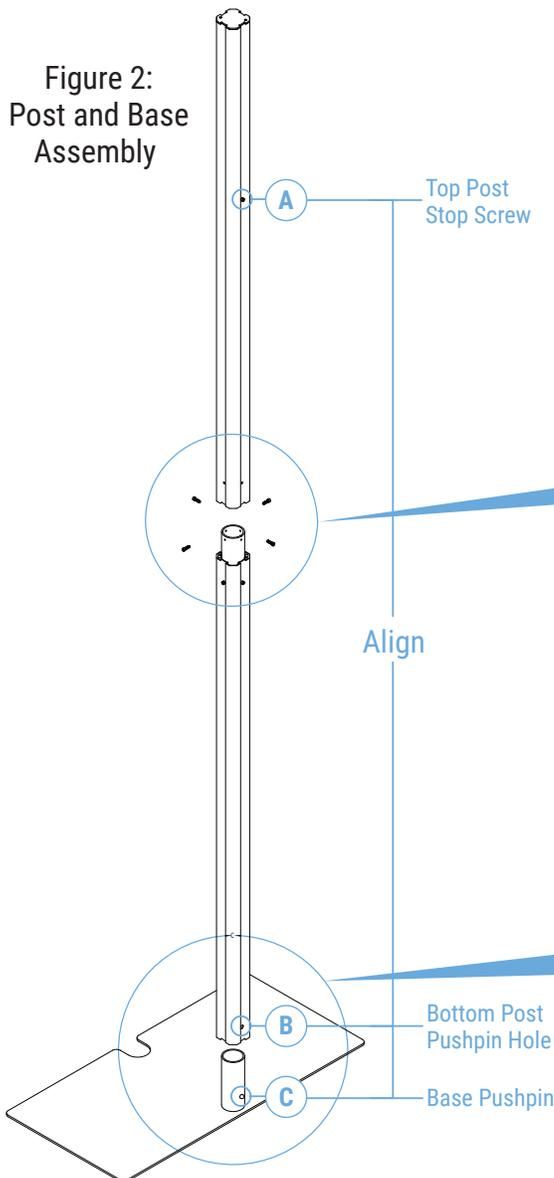
**1** Connect post top and bottom while aligning top post stop screw (A) and bottom post pushpin hole (B).
