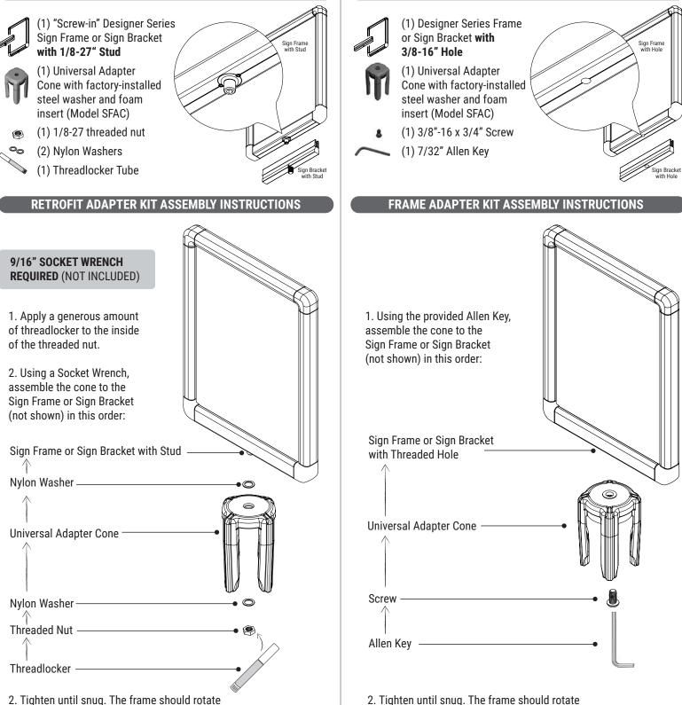
for orientation when installed on the post.
