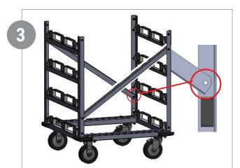
Install 37" Long Diagonal Bars connecting both Side Frame Walls, ensuring that the flat edge nests into the corners of the Side Frame Wall so holes line up properly.
