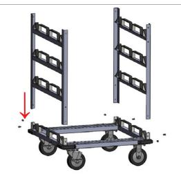
Turn unit over onto wheels. Align Side Frame Walls with Post Holder Brackets on Cart Base and install M8x1.25–15mm Long Bolts with Lock Nuts.
