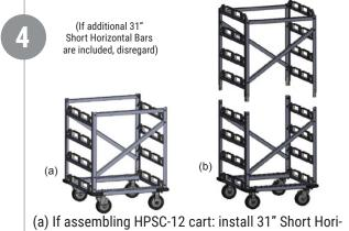
(a) If assembling HPSC-12 cart: install 31" Short Horizontal Bars to connect the top of the Side Frame Walls.
