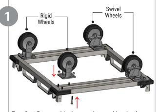
Turn Cart Base upside-down and assemble wheels with M10x1.5-60mm Long Bolts with Lock Nuts. Note location of Swivel and Rigid Wheels-(1) Swivel Wheel and (1) Rigid Wheel on each rail.
