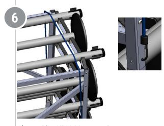
If assembling HPSC-24 cart, use Bungees to secure top posts by inserting bungee hook end into holes mid-way up the cart.
